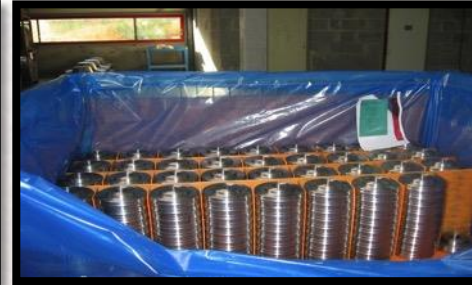
Application for Anti-Corrosive VCI Material
