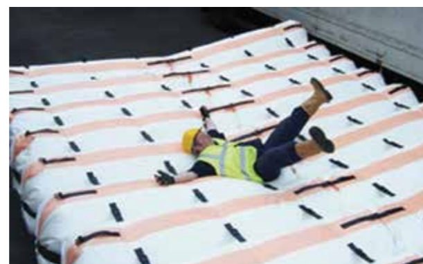
Fall Arrest Systems (below) like airbags, from our Advanced Composite division, are used in health and safety applications.
